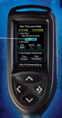
Use the SELECT button when a box is—highlighted to edit the values. Once the digit is highlighted in yellow, use the UP and DOWN buttons to increase or decrease the number. Press SELECT again to accept the value and move to the next digit or field.
