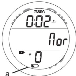
Fig. 3 - LOW BATTERY WARNING
