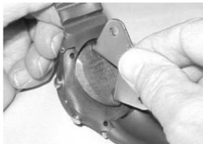
Fig. 112A - BATTERY HATCH REMOVAL (Tool)
