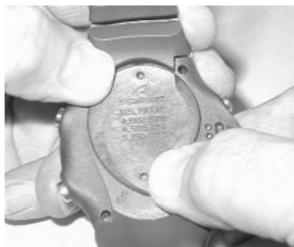
Fig. 112B - ALTERNATE HATCH REMOVAL
