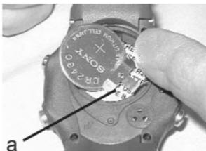
Fig. 113 - BATTERY REMOVAL
