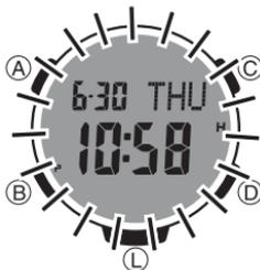
The display of the dive computer is illuminated for easy reading in the dark. The dive computer's auto light switch turns on illumination automatically when you angle the dive computer towards your face.
