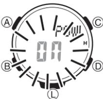
1. In the Time mode or Surface Mode, hold down **A** for at least 2 seconds. First, SET Hold will blink on the display, and CITY will be displayed in the upper right display. After that, the currently selected city code and city name will scroll across the upper right display. Keep **A** depressed until the scrolling starts.
