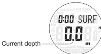
In addition, if after switching to Free diving mode, you do not dive in water of depth 1m or more for 60 minutes or more, the unit automatically returns to Time mode. In addition, the unit does not return to Time mode when you press the B)MODE button when you are diving a depth of 1m or more, but will stay in Free diving mode. However, if it continues for over 99 minutes, the unit returns to Time mode.
