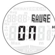
5. By pressing A) ADJUST button twice, after passing through the Depth interval alarm settings screen, the unit switches to fixed display of Gauge mode ON. Press and hold the B) MODE button (for about 2 seconds) and the unit switches to Time mode. In addition, the unit switches to Time mode if left for about three minutes.
