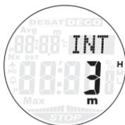
4. Press the D) PLAN mode button to increase the water depth in increments of 1m or press C) LOG button to decrease the water depth. Press the B) MODE button to switch the setting ON or OFF.
