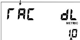
Figure 33a PROGRAMMING MODE (Setting TACLITE On Time)
