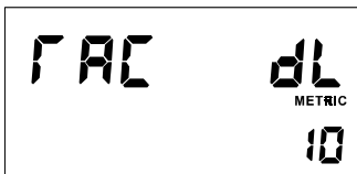
Figure 33 PROGRAMMING MODE (Setting TACLITE On Time)
