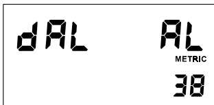
Figure 25 PROGRAMMING MODE (Setting Depth Alarm)
