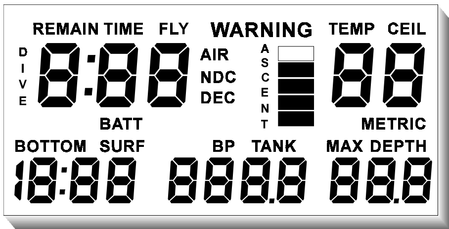
Fig-1 Self-Diagnostic Mode
