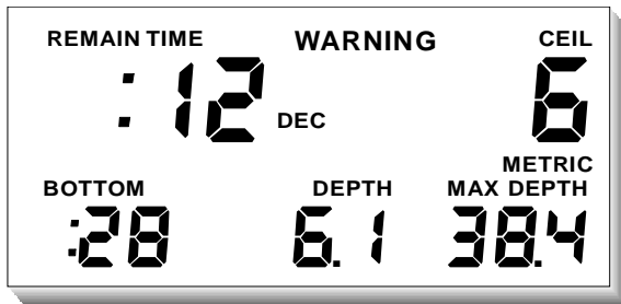
Figure 7 DECOMPRESSION MODE (Showing TotalDeco Time)
