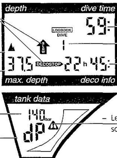
The diagram shows the Aladin Air X dive computer display. It is divided into several sections: 'depth' (showing 37.5), 'dive time' (showing 59:), 'LOGBOOK DIVE' (showing 1), 'DECOSTOP' (showing 22 h 45:), 'max. depth', 'deco info', and 'tank data' (showing 140 bar and dP). A hand icon points to the 'LOGBOOK DIVE' section. A warning icon points to the 'dP' section.
