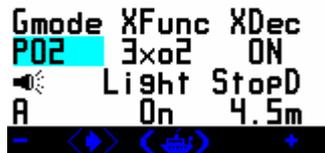
Xfunc = 3xo2. This turns on the option. Once turned on, then XDec can be enabled, and Gmode can be chosen as PO2.
