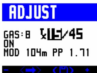
Move the cursor to select your chosen calibration gas, either Air in your gas list and switch it ON
