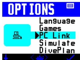
In the OPTIONS screen a short push of the left switch moves the highlight downwards. A long push on the left switch moves the highlight upwards.
