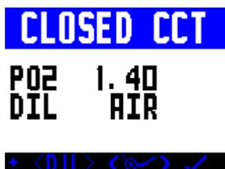
Entering this mode allows the selection of a closed circuit decompression algorithm and opens a CLOSED CCT screen. In this screen the gas mix you have selected is displayed as a diluent (DIL). Change the diluent as required by a short push of both switches then following the same procedure as outlined above for selecting and adjusting an open circuit gas.
