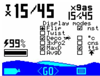
Enabling the Display modes 3xPo2 option displays all three cell values in the dive screen.
