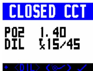
Make sure you are in Closed Circuit Mode and you see CLOSED CCT at the top of your screen if not, go to Closed Circuit mode by a long push on both switches.
