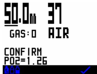
In this screen a long push of the left switch will take you into the Gas SELECT and ADJUST screens and add a gas, change the parameters of a gas or switch a gas on or off just as you could on the surface.
