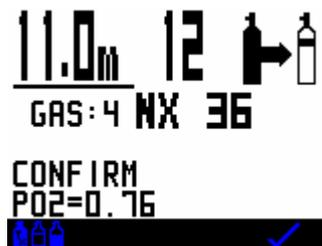
This will take you into a screen where you will see the gas switch symbol and the new gas you have just switched to. A short push on the right switch will then take you back into the dive screen where the new gas will be displayed and decompression will begin to be calculated based on this gas.
