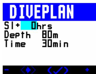
Once you have set your planned dive gases in the VR. Diveplan allows you to enter depth, time and surface interval and calculate a set of backup tables.
