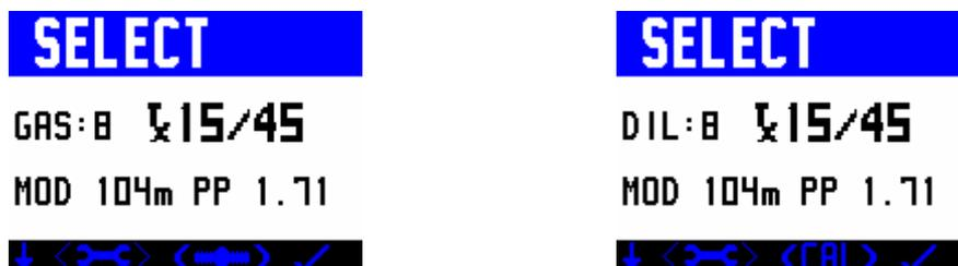
In the gas SELECT screen, short pushes on the left-hand switch take you through the ON gases. Up to 10 gases are available for selection (G10 mode). Simply keep pressing until the gas you wish to breathe at the start of the dive is displayed. Once you are confident that the correct gas is indicated, a push of the right switch will confirm. Your selected gas will now be displayed in the centre of the Home screen (or the DIVE screen if you are diving).
