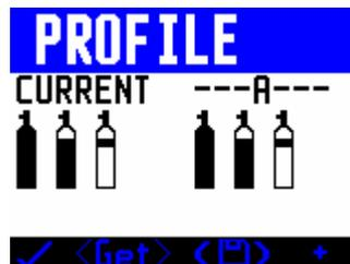
A short push of both switches in the GAS LIST screen takes you to PROFILE which you can use to programme sets of gases, as follows.
