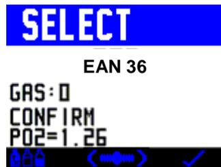
This will take you into a screen where you will see the new gas you wish to switch to based on the MOD of that gas and the plan you entered. A short push on the right switch will then take you back into the dive screen where the new gas will be displayed and decompression will begin to be calculated based on this gas.
