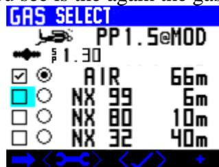
When you exit this screen, you have the option to change the PO2's as already described using a short push of + for small changes or a long push of + to toggle to the previously saved PO2.
