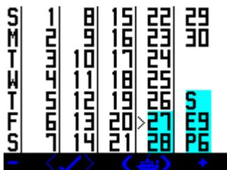
A short push on + or - moves the marker back and forward one day. A long push moves 30 days. Days with dives are highlighted.
