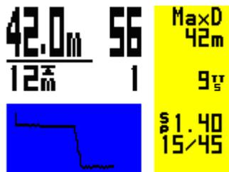
If XDec is set to YYY and XFunc is set to 3xO2 then all three sensors and the average PO2 (x1.15) will be displayed. An x (x1.15) denotes that the external cell reading is being used.
