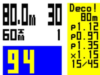
Note: if the partial pressure of oxygen in the diluent at the prevailing dive depth exceeds the DG05's internal set point, then the diluent PO2 will be displayed instead of the set-point.
