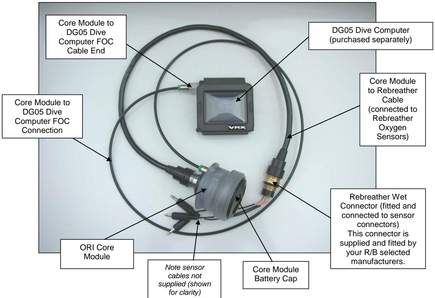
**NOTE:** Hollis Gear can supply the rebreather wet connector to rebreather manufacturers and approved service centres **ONLY**. They will fit and test the connector and ensure the correct interfacing to the rebreather's existing control system. The core module to rebreather cable then simply plugs into the fitted wet connector.
