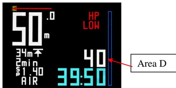
The OLED screen has an additional option. Area D will change in conjunction with GMode as per the table except it does not generate a graph mode and will show TTS instead.
