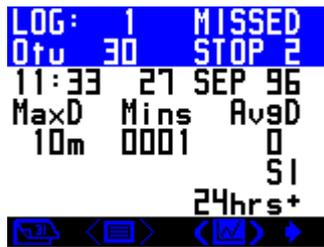
The logbook screen shows depth, time and surface interval information as well as accumulated OTUs (oxygen tolerance units). If a decompression stop is missed or violated during a dive, the MISSED STOPS warning is displayed in the top right corner of the screen. If multiple stops have been missed, the number of stops missed is shown immediately after the word STOPS.
