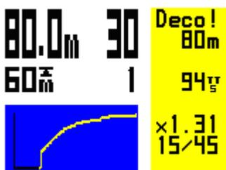
In closed circuit mode with an external cell connected and XO2 set and XDec ON the actual from the external cell PO2 is shown on the second line up.
