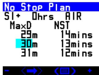
In this screen you can see No Stop Times (NST) for depths to 41m, taking into account your previous dives and surface interval. The surface interval and target depth are user changeable. Note that the surface interval figure that you set is in addition to time already spent out of the water. When using the Buhlmann algorithm, you may be surprised that the No Stop times appear to be short. They do in fact correspond to standard Buhlmann dive tables which incorporate safety stops.
