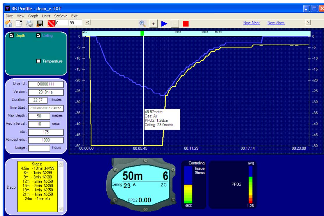
The decompression information is shown in the bottom left corner of the dive display window. When there are stops, the window background is set to yellow.
