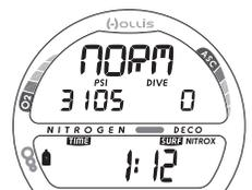
Fig. 17 - NORM SURF MAIN (no dive made yet)
