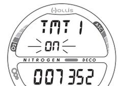
Fig. 48 - SET TMT 1 (On/Off, then Code)
