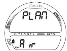
Fig. 21A - PLAN LEAD-IN (AIR)
