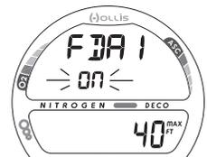
Fig. 100A - SET FREE DEPTH ALARM
