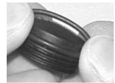
Fig. 118 - TRANSMITTER O-RING INSTALLATION
