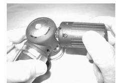
Fig. 121 -INSTALLING A TMT ON A REGULATOR
