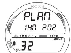
Fig. 21B - PLAN LEAD-IN (Nitrox)
