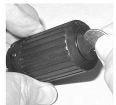
Fig. 115 - TMT BATTERY COVER REMOVAL
