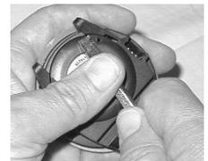
Fig. 112 - COVER REMOVAL (using screwdriver)
