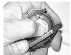
Fig. 113 - COVER REMOVAL (using spanner tool)
