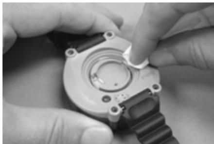
5. Using a clean, dry, lint-free cloth, wipe the sealing area of the battery compartment. Inspect to make sure it is completely clean and dry.
