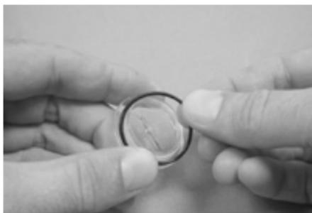
2. Using your fingers, remove the O-ring from the battery hatch and discard. Do not use any tools to remove the O-ring.
