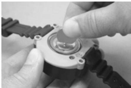
1. Using a coin (never use a screwdriver), turn the battery hatch counter clockwise and remove it from the case.
