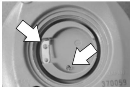
4. Inspect the gold contact and small spring contact for signs of bending, breakage or corrosion. If you find any signs of damage, return the unit to your authorized dealer and do not attempt to use it.
