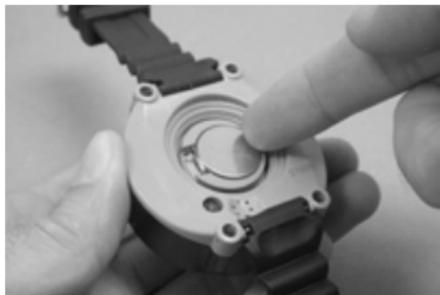
3. With your finger, lift up on the edge of the battery opposite the gold contact and remove the battery.
