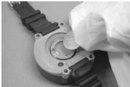
7. Lightly lubricate a new O-ring using a food-grade silicone grease, such as Dow Corning 111. This grease is available at most dive shops. Do not overlubricate. Install the new O-ring onto the battery hatch. Carefully thread the battery hatch into the case in a clockwise direction until snug. Using a coin, tighten the battery hatch until it can no longer be turned.
