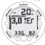
PLONGEE AVEC PALIER DE DECOMPRESSION, AU-DESSUS DU PLAFOND. UNE FLECHE POINTEE VERS LE BAS, UN SIGNAL ER ET UNE ALARME. VOUS DEVEZ IMMEDIATEMENT (DANS LES 3 MINUTES) DESCENDRE AU PLAFOND OU PLUS BAS.
