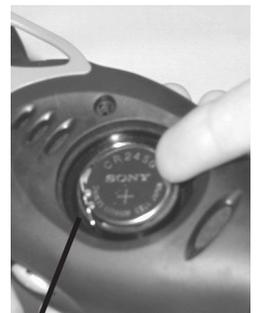
a Fig. 90 - Battery Installation
