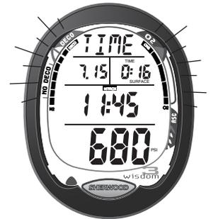
Fig. 86 - Gauge Mode on Surface
