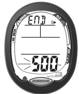
Fig. 45 - Set End Pressure Alarm Value
