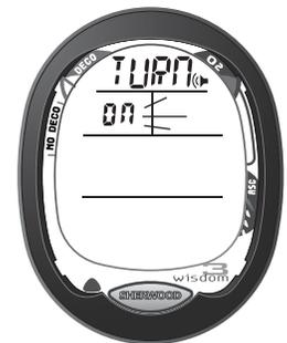
Fig. 42 - Set Turn Pressure Alarm
