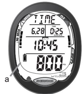
Fig. 8 - Low Battery Condition
