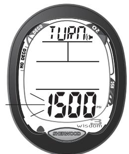
Fig. 43 - Set Turn Pressure Alarm Value
