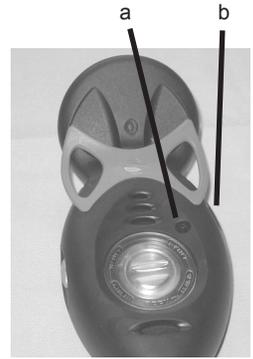
Fig. 87 - Depth Sensor & Data Port
