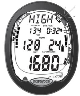
Fig. 74 - High PO2 Alternate
