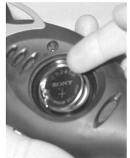
Fig. 89 - Battery Removal
