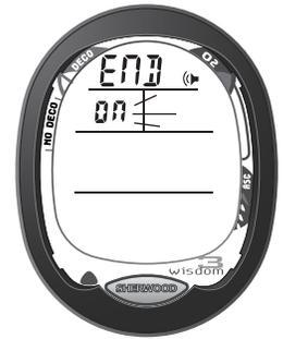
Fig. 44 - Set End Pressure Alarm
