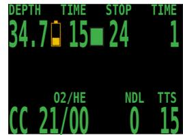
Across the top line is the title for the first row of information. This area only changes during the display of the dive log. The first data area shows depth, battery warning, dive time, ascent rate, first stop depth, and first stop time. It is showing a depth of 34.7 meters, a low battery alarm, 15 minute dive time, a 3 meter per minute ascent rate, and a stop at 24 meters for 1 minute.
