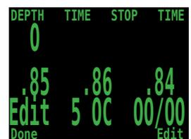
Only enter the gases you are actually carrying on the dive. With radio station gases, the computer has a full picture of the OC and CC gases you are carrying and can make informed predictions about decompression times. There is no need to turn gases off and on when you switch from CC to OC, because the computer already knows what the gas sets are. You can still add or remove a gas during the dive if needed.
