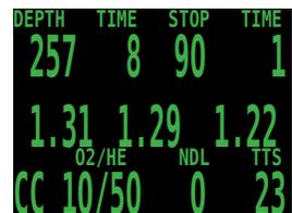
The diver is ascending to the 90 foot stop. Note the ascent rate indicator showing a 30 fpm / 10 mpm ascent rate. Although the ascent rate is 30 fpm now, during the 7 minute ascent, the diver ascended slower than was predicted, and now there is a 100 foot stop.
