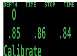
Pressing the MENU button will prevent the calibration. Pressing SELECT will calibrate the sensor displays. The displays should now all read .98. If any display shows **FAIL**, the calibration has failed because the mV reading is out of range.
