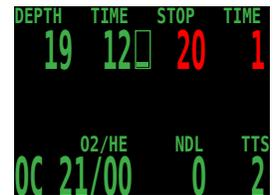
As we ascend, the ascent rate indicator shows about 30 fpm or 9 mpm. When we approach the first stop, our ascent rate slows to about 10 fpm and when we go shallower than our first stop, the stop depth starts to flash red.
