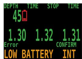
This alarm appears when the voltage on the external solenoid battery is low (controller only). The solenoid may still be firing, but the battery must be replaced before any further diving.
