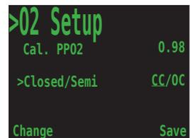
It also allows SCR divers to set their calibration percentage to .21. Note: When in semi-closed mode the user cannot utilize internal monitoring.
