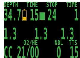
The next area is the title for the bottom line. This title changes frequently in the menu system to provide additional information about the bottom line. The last line shows that the computer is in closed circuit (CC) mode with a gas containing 21% oxygen and 0% helium.
