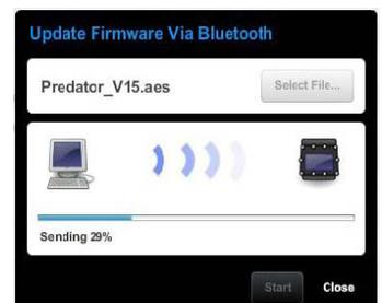
The Predator screen will give percentile updates of receiving the firmware, then the PC will read "Firmware successfully sent to the computer".
