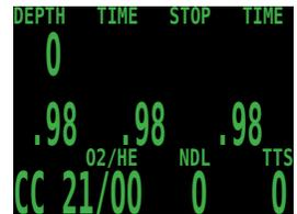
Next, we check the closed circuit gases that we have programmed. Entering the gas selection function by pressing SELECT with the "Select Gas" menu item showing will display the first CC gas that is available. MENU will increment to the next gas available. Another MENU takes us back to the "Select Gas" menu item. Those are the only two gases configured. We SELECT gas number 2, the Trimix 10/50.
