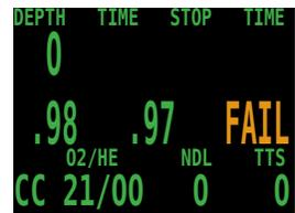
If this was the display, it would indicate a faulty sensor. It is not within the normal range for a sensor in oxygen. Most sensors are designed to output 10 mV +/- 3 mV in air. If the output is linear, then that translates to a range of 30 to 70 as valid mV readings in 98% oxygen. The computer will refuse to calibrate outside that range.
