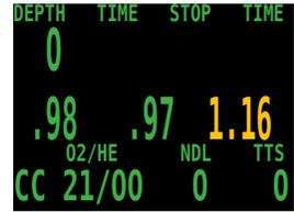
A failed sensor is a different situation. In this case, the sensor failed calibration. Changing the sensor won't make it register again. Once a sensor has failed calibration, the only way to bring it back is to successfully calibrate. If the computer were to display a value with a new sensor, it would be a meaningless value without calibration.
