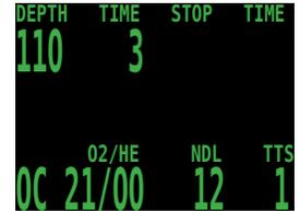
As the dive starts, the depth increases. The display is showing the computer programmed for open circuit (OC) air.
