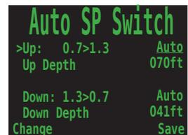
The next option is still a part of the switch up function, and enables the editing of the switch depth.
