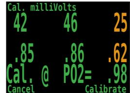
The system defaults to a calibration gas of 98% oxygen. This is to compensate for the difficulty in completely filling the loop with 100% oxygen and also to allow for water vapour. If you are using a calibration kit with no water vapour and 100% O<sub>2</sub>, you can set the calibration gas to 100. It can also be set to other values if pure oxygen is not available.
