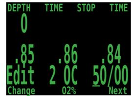
Each push of the MENU button will increment the digit being edited. When the digit reaches 9, it will roll over to 0.
