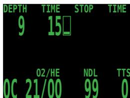
When we clear the last stop, the stop depth and time goes blank, and now we see a NDL of 99 minutes again. Once we surface, the depth is 0 and a minute later when the computer comes out of dive mode, the NDL goes to 0 as well.
