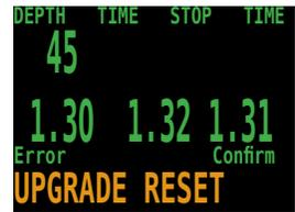
This error usually occurs when the battery dies while the computer is asleep. If the battery gets too low to maintain system integrity, the hardware will force the system into reset.
