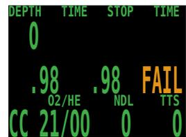
The calibration takes into account the altitude at which the computer was turned on. For example, if the altitude was 885 mBar or .87 ATA, then with a 98% calibration gas, the sensors would calibrate to .85.
