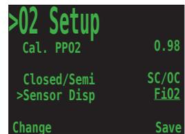
In Semi-Closed mode you have the option of displaying the partial pressure of oxygen (PPO2) or the fraction of inspired oxygen (FiO2) for the three oxygen sensor displays in the default screen.
