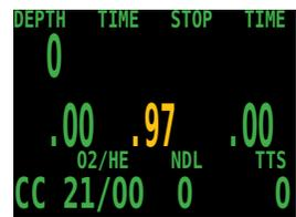
With sensors one and three unplugged, we simulate the situation with fourth sensor monitoring. If we calibrate in this situation, the system will assume that this computer is only attached to one sensor, and will re-configure for fourth sensor monitoring.
