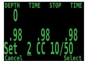
The system will use both of these gases for our dive when calculating the TTS. It assumes a diluent switch at a PPO2 of 1.0. That means that it will assume that you have switched to an air diluent at 124 feet. This is only for TTS. The computer will always use the currently selected gas for tissue loading calculations.
