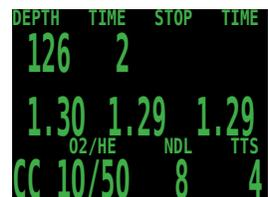
The computer has automatically switched to the high setpoint. This can be disabled if automatic setpoint switching isn't required.
