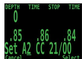
When the system is not in a menu, pushing SELECT will bring up information displays with various dive status information. This is the first information display showing the diluent PPO2 amount, the current CNS loading, the setpoint (if applicable), and the average PPO2 being used for decompression calculation.
