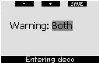
During the dive, if you are about to enter decompression and the warning is set to either **VISUAL** or **BOTH**, Galileo will show the message **ENTERING DECO** on the display for 12 seconds. The following figures show the actual display in the **CLASSIC**, **LIGHT** and **FULL** configurations.
