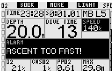
Galileo also provides an audible alarm in case of ascent rates exceeding 110%: the intensity of the alarm increases in direct proportion to the degree that the ideal ascent rate is exceeded.
