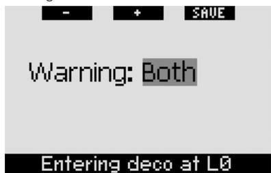
During the dive, if you are about to enter decompression and the warning is set to either **VISUAL** or **BOTH**, Galileo will show the message **ENTERING DECO AT L0** on the display for 12 seconds. The following figures show the actual display in the **CLASSIC**, **LIGHT** and **FULL** configurations.
