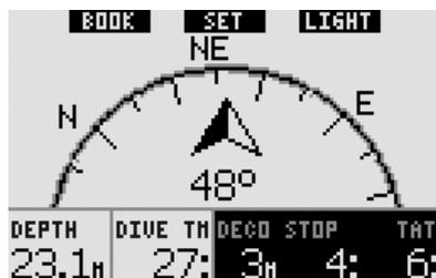
In this lay-out, the button functions change slightly. The middle button is now marked **SET**. **Pressing** this button will set the bearing. Compass bearing represents the direction the front of the computer is pointed at. It is expressed in degrees, from 0 to 359. 0 degrees is North, 90 degrees is East, 180 degrees is South, 270 degrees is West and any other reading is interpolated in between.
