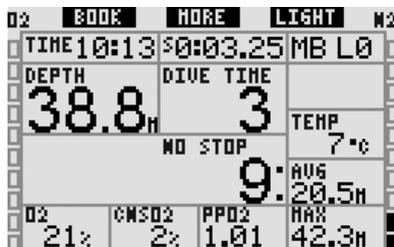
Galileo also has a gauge mode, with a corresponding **GAUGE** configuration, in which the computer acts as a digital depth gauge and does not perform any decompression calculation.
