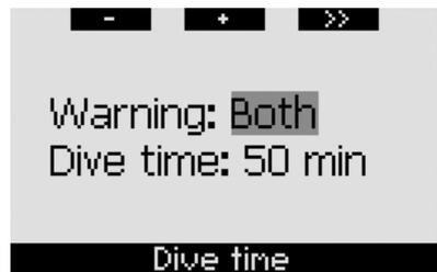
During the dive, if the dive time reaches half the value of the set dive time and the warning is set to either **VISUAL** or **BOTH**, Galileo will show the message **TURN-AROUND TIME** on the display for 12 seconds. The following figures show the actual display in the various dive configurations (**CLASSIC**, **LIGHT** and **FULL**).
