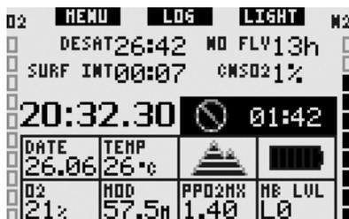
You should not undertake a dive as long as the no-dive warning is displayed on the computer screen. If the warning is prompted by microbubble accumulation (as opposed to CNS O<sub>2</sub> over 40%) and you dive anyway, you will have shorter no-stop times or longer decompression times. Moreover, the duration of the microbubble warning at the end of the dive can increase considerably.
