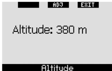
To set the altitude, first **press ADJ** to enter the **ADJUST ALTITUDE** menu. Once inside this menu, use the **+** or **-** buttons until you reach the desired value. Each time you **press +** or **-**, the displayed altitude will change in 10m/50ft increments. **Press SAVE** to confirm your choice and return to the main **Altimeter** menu.
