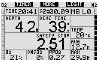
In compass mode, the safety stop timer works the same way as in the **CLASSIC**, **LIGHT** and **FULL** configurations. If the safety stop timer is active while switching from one configuration to the other, the timer information itself will transition smoothly between displays.
