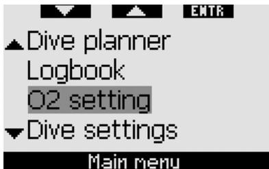
To change settings **press** the + or - buttons, then **press SAVE** to confirm the changes. This will take you back to the main menu. If you do not want to confirm the changes, **press and hold** the right button at any time to exit without saving the changes. This will also take you back to the main menu. **Press and hold** the left and the right button simultaneously to jump back to the **time of day** display. Note that holding down the + or - buttons makes the setting change faster.
