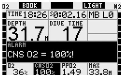
In all configurations, the alarm message and the audible signal are repeated for 5 seconds in one minute intervals after the first occurrence and for as long as the value of CNS O<sub>2</sub> stays at or above 100% or until the ppO<sub>2</sub> drops under 0.5bar (see section 3.1 for a list of depths at which ppO<sub>2</sub> equals 0.5bar for some typical Nitrox mixes).
