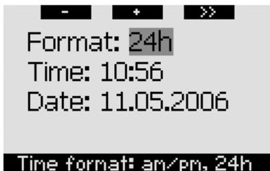
Pressing **SAVE** at the last setting starts the clock at the set time and zero seconds.
