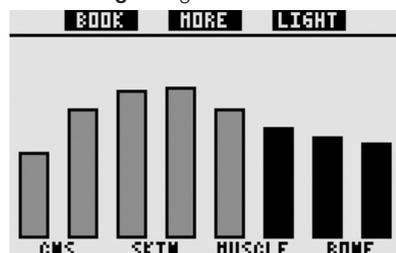
If you have uploaded pictures onto Galileo, you can view them during the dive by **pressing MORE** while the individual compartment saturation is displayed. Every time you **press MORE** while a picture is showing, the next picture in the memory sequence of Galileo will be called up. Each picture stays on the screen for a maximum
