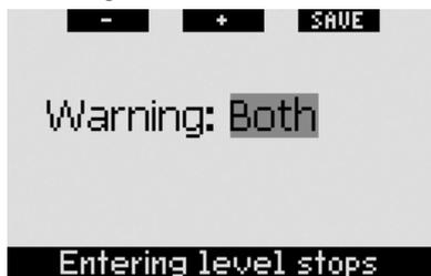
During the dive, when you are about to enter the level stop phase and the warning is set to either **VISUAL** or **BOTH**, Galileo will show the message **ENTERING LEVEL STOPS** on the display for 12 seconds. The following figures show the actual display in the **CLASSIC**, **LIGHT** and **FULL** configurations.
