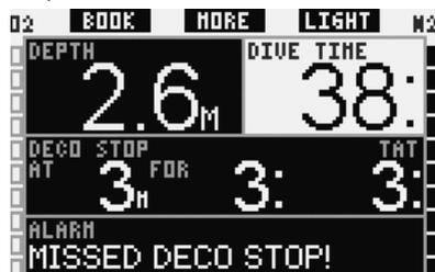
In **LIGHT** configuration, in presence of a missed decompression stop, the display momentarily switches to the **CLASSIC** configuration, and the alarm is presented as described above. Once the diver returns to the prescribed depth, the displays resumes the **LIGHT** configuration.
