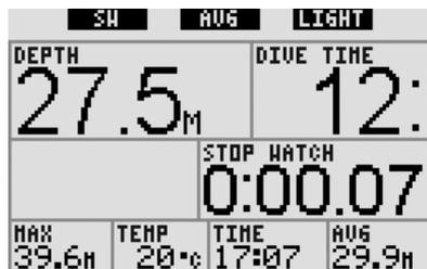
For all three configurations and in gauge mode it is possible to call up the digital compass at any time during the dive. It is also possible to rotate the entire screen by 180 degrees, so that the computer can be worn with the buttons on the top or on the bottom.
