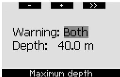
During the dive, if you descend below the set depth and the warning is set to either **VISUAL** or **BOTH**, Galileo will show the message **MAX DEPTH REACHED** for 12 seconds in place of the no-stop or decompression information.
