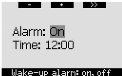
This menu allows you to set a wake-up alarm. The time of the alarm is shown in the format specified in the **Time** menu (either in **AM/PM** or **24hour**). When the alarm is set to **ON**, a bell symbol appears in the **time of day** display.
