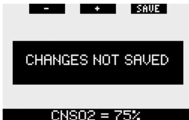
If more than one entity can be changed within a single menu, the right button is labeled >> instead of **SAVE**. **Pressing >>** will move the highlighted segment to the next entity that can be changed. When the highlighted segment is on the last possible entity that can be changed, the right button reverts back to **SAVE**. In case of submenus, the operation follows the same process.
