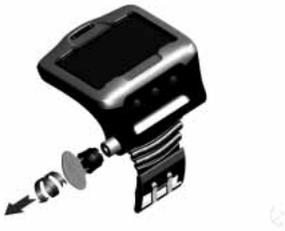
3. Inspect the o-ring on the battery cap. If you see traces of seeping water, damages or defects on the o-ring, replace the o-ring with an original UWATEC replacement part (PN 06.202.693). The o-ring is provided with the UWATEC battery kit for Galileo (PN 06.202.872). When replacing the o-ring, make sure the new o-ring is in perfect condition and well lubricated, and that the o-ring, o-ring groove and sealing surfaces are free of dust and dirt.
