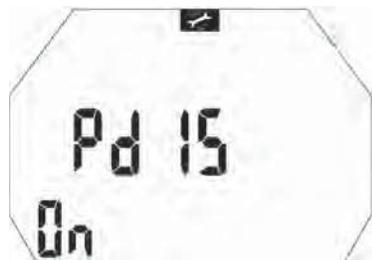
1. Confirm that you wish to enable PDIS by pushing  . "On" or "off" starts to flash.
