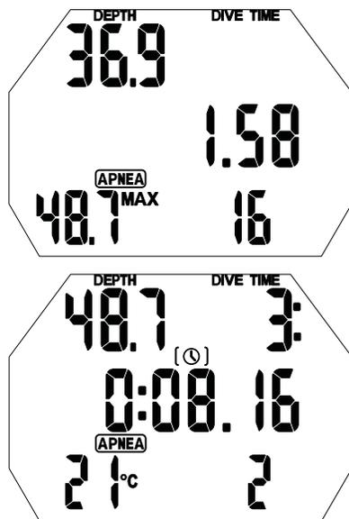
In Apnea mode the dive can be started manually by pressing  $\circ \bullet$ . This function allows fast sampling to start straight from the surface. Automatic start of the apnea dive will happen from depth of 0.8m/3ft. Once activated the Apnea mode will run 15 minutes after surfacing. This allows you to start a repetitive apnea dive with precise data in the logbook. Surface mode can be stopped with long press  $\circ \bullet$ .
