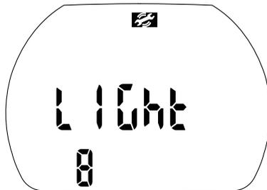
1. Confirm that you wish to change the duration of the backlight illumination by pushing   . The value starts to flash.
