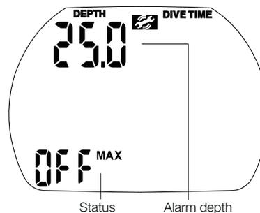
1. Confirm that you wish to change the depth of the alarm or to switch it on or off by pushing  $\odot \bullet$ . The depth starts to flash.
