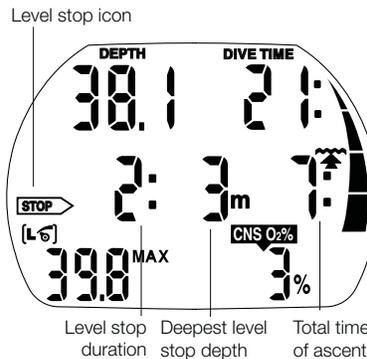
On entering the level stop phase, "NO STOP" disappears and the arrow appears. The arrow flashes for 8 seconds and an audible attention beep goes off. To complete the dive without cascading to a lower MB level, all requested level stops must be observed.
