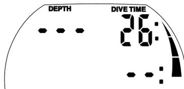
At a diving depth of less than 0.8m (3ft) the display shows "----".
