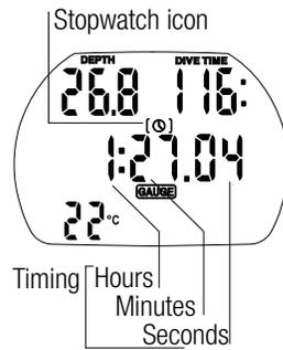
In gauge mode, after immersion, Aladin 2G will automatically monitor the dive time and at the same time activate the stopwatch. The stopwatch will run for a maximum of 24 hours.
