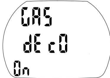
1. Confirm that you wish to enable two-gas diving by pushing  . "On" or "off" starts to flash.
