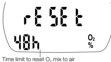
1. Confirm that you wish to change the time limit of the reset by pushing  $\odot \bullet$ . The current setting starts to flash.
