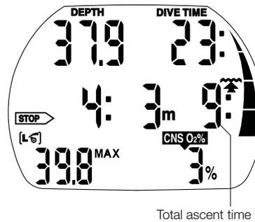
Aladin 2G displays the level stop information and the total time of ascent. This includes the time of ascent as well as all level stops.
