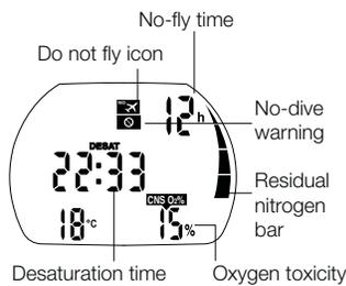
From the **time of day display** you can check the desaturation time\* by pushing . Desaturation time is determined either by oxygen toxicity, nitrogen saturation or the regression of microbubbles, depending on which requires the longer time.
