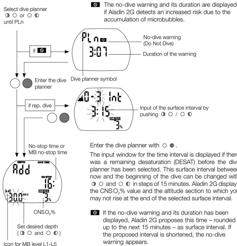
Confirm the displayed interval with  $\odot$   $\bullet$  (if applicable).
