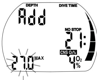
Confirm the desired depth with  $\odot$   $\bullet$
