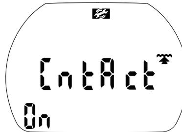
On submerging in water the water contacts switch on Aladin 2G automatically.
