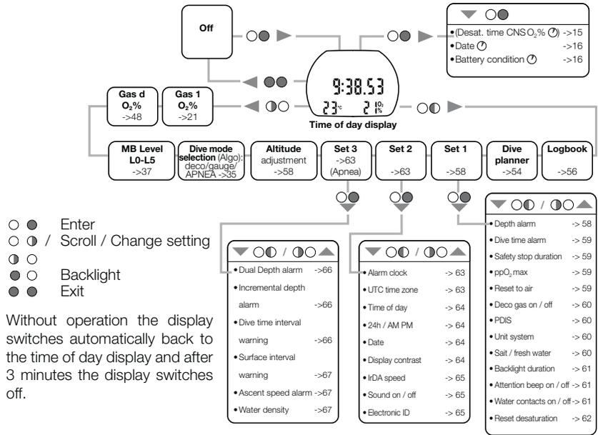
Without operation the display switches automatically back to the time of day display and after 3 minutes the display switches off.
