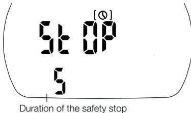
1. Confirm that you wish to change the duration of the safety stop by pushing  $\odot \bullet$ . The duration starts to flash.
