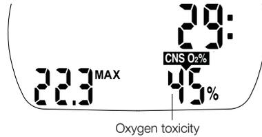
Aladin 2G calculates oxygen toxicity based on depth, time and the gas mixture and displays it in the location of the ascent rate. The toxicity is expressed in 1% increments of a maximum tolerated value (O<sub>2</sub> clock). The symbol "CNS O<sub>2</sub>" is displayed together with the percentage.
