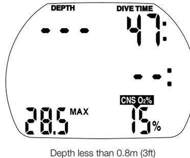
After reaching the surface (<0.8m/3ft) Aladin 2G remains in dive mode for 5 minutes. The delay allows for surfacing for a short period for orientation.
