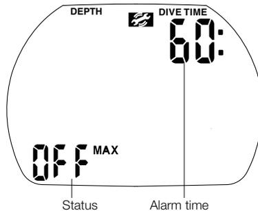
1. Confirm that you wish to change the time of the dive time alarm or to switch it on or off by pushing  $\odot \bullet$ . The alarm time starts to flash.
