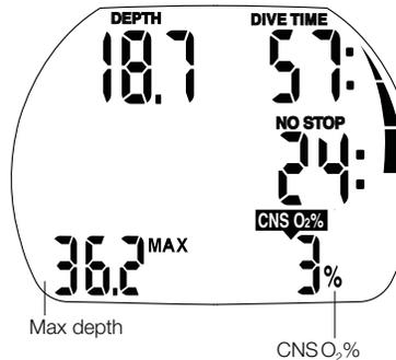
Max depth is only displayed if it exceeds the current depth by more than 1m (3ft) (maximum indicator function). If max depth is not displayed, Aladin 2G shows the temperature.
