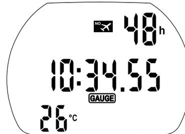
Remaining time during which Aladin 2G cannot be used in computer mode
