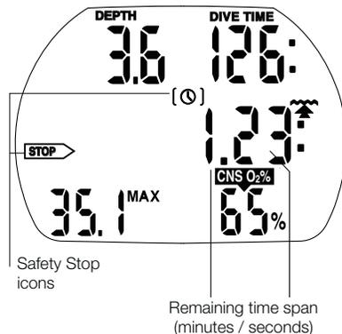
The safety stop timer displays the time span a diver should spend at the safety stop depth at the end of the dive. The timer starts automatically when depth is shallower than 6.5m and counts back from 3 minutes (default) to zero. It can be restarted manually any number of times. The duration of the timer can be set between 1 and 5 minutes.
