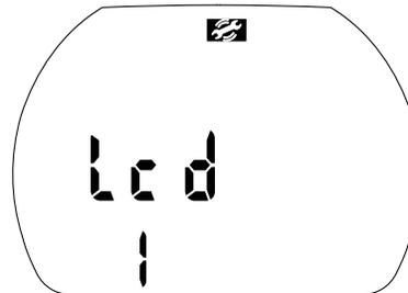
1. Confirm that you wish to adjust the display contrast by pushing   . The current setting starts to flash.
