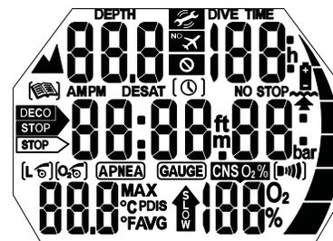
Switch on Aladin 2G by pushing  $\odot$   $\bullet$  and check the test display: Are all elements of the display activated? Do not use Aladin 2G if the display does not show all elements. When switching on Aladin 2G with  $\odot$   $\bullet$ , the test display will not appear.
