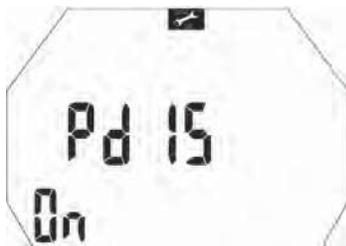
When the calculated PDI stop is deeper than 8m/25ft, Aladin 2G shows it on the display and continues to do so until you reach the displayed depth during an ascent. The displayed value changes during the dive as Aladin 2G tracks the uptake of nitrogen in the 8 compartments
