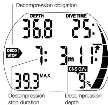
On entering the decompression phase, "NO STOP" disappears, the DECO STOP symbol appears and an attention beep goes off. The nitrogen loading bar stops flashing and the 6<sup>th</sup> segment lights up (red area). The deepest decompression stage in metres (feet) is displayed and the decompression
