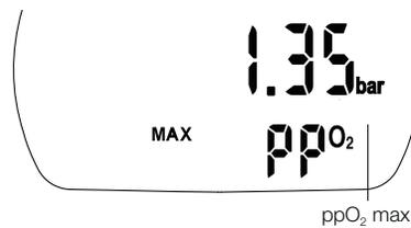
1. Confirm that you wish to change the ppO<sub>2</sub> max by pushing  $\odot \bullet$ . The current value starts to flash.
