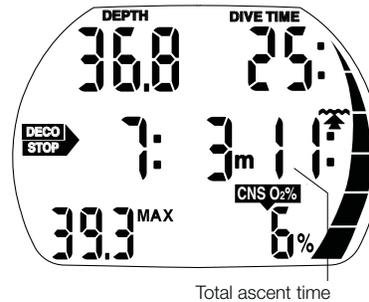
As soon as decompression stops are necessary Aladin 2G shows the total time of ascent. This includes the ascent time from the current depth to the surface and all decompression stop obligations.
