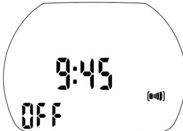
The alarm clock goes off only at the surface. “Sound” must be turned “on” in “set 2”.
