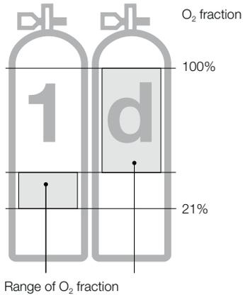
During dives with two gas mixtures the bottom mix (gas 1) contains the lower fraction of oxygen. Aladin 2G will only accept settings corresponding with this order.
