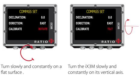
For a correct survey, carry out the calibration far from magnetic field sources i (PC, TV, light poles etc.)
