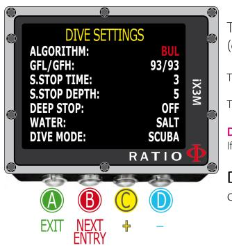
**S. STOP TIME:** It sets the Safety Stop's time in minutes. You can set the time from 0 to 9 minutes (if 0 the Safety Stop is omitted)
