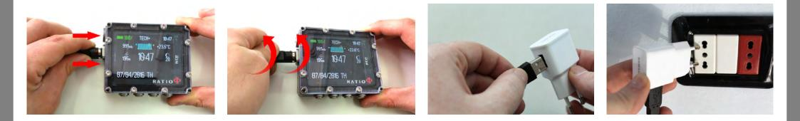
To recharge the RATIO iX3M we recommend to use a wall USB plug (like the one of your mobile/tablet). If you decide to use a PC USB plug (deprecated), make sure that the PC doesn't interrupt the electricity flow once in stand-by.
