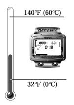
Fig. 22 - Operating Temperature Range
