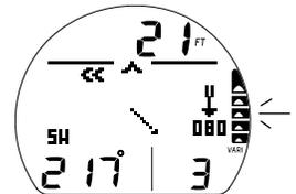
Fig. 127 – ALARME DE REMONTÉE
