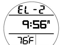
Fig. 8 – ÉCRAN SECONDAIRE ALT 2 DU MODE SURFACE NORM
