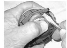
Fig. 138 – AJUSTEMENT DE LA BAGUE DE FIXATION DU COUVERCLE
