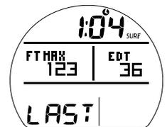
Fig. 7 – ÉCRAN SECONDAIRE ALT 1 DU MODE SURFACE NORM
