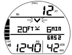
Fig. 56 – ÉCRAN PRINCIPAL D'INFRACTION PROVISOIRE
