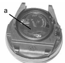
Fig. 136 – PILE DU VT 4.0 INSTALLÉE
