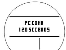
Fig. 131 – CÂBLE D'INTERFACE PC CONNECTÉ
