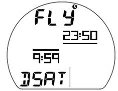
Fig. 10 – FLY/DESAT (INTERDICTION DE VOL/ DÉSATURATION)
