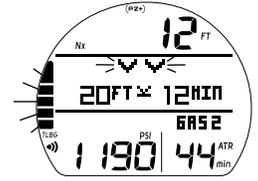
Fig. 57 – ÉCRAN PRINCIPAL D'INFRACTION DIFFÉRÉE 1 (pendant signal sonore)
