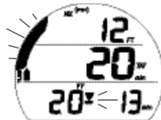
Fig. 67 - ÉCRAN PRINCIPAL D'INFRACTION DIFFÉRÉE 1 (pendant signal sonore)
