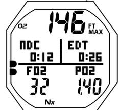
Fig. 94 - ÉCRAN SECONDAIRE D'ALARME PO<sub>2</sub>
