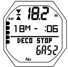
Fig. 84 - ÉCRAN PRINCIPAL D'INFRACTION DIFFÉRÉE 2
