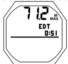
Fig. 90 - ÉCRAN SECONDAIRE D'INFRACTION AVEC LIMITATION AU MODE PROFONDIMÈTRE
