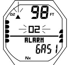
Fig. 98 - ÉCRAN PRINCIPAL D'ALARME DE HAUT NIVEAU D'O<sub>2</sub> (100%)
