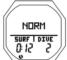
Fig. 92B - ÉCRAN PRINCIPAL SURFACE D'INFRACTION AVEC LIMITATION AU MODE PROFONDIMÈTRE
