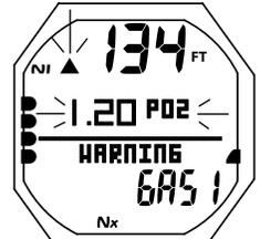
Fig. 93A - MISE EN GARDE PO<sub>2</sub> (pendant signal sonore)
