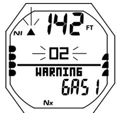
Fig. 97 - AVERTISSEMENT DE HAUT NIVEAU D'O<sub>2</sub> (80%) (pendant signal sonore)
