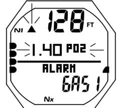
Fig. 93B - ÉCRAN PRINCIPAL D'ALARME PO<sub>2</sub>
