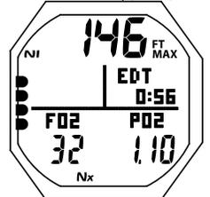
Fig. 99 - ÉCRAN SECONDAIRE D'ALARME O<sub>2</sub>
