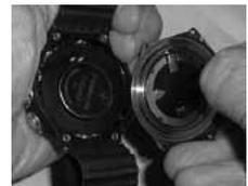
Fig. 166B - SOULEVER POUR RETIRER LE COUVERCLE DE LA PILE
