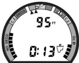
Fig. 32 - Main Display (Alt On)
