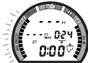
Fig. 60 - Delayed Violation (deeper than 330ft/99.5m)
