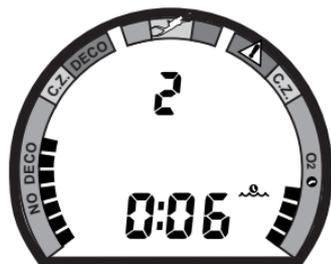
Fig. 38 - Post Dive Surface Mode (< 10 min)
