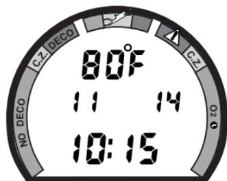
Fig. 39 - Temperature/Date/Time
