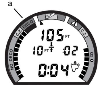
Fig. 35 - Entering Into Decompression Mode
