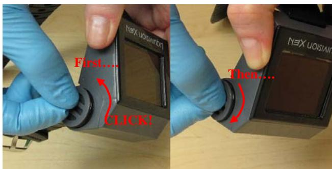
Screw the battery cap on the compartment using your fingers. NEVER overtighten the battery cap. Use your fingers, NEVER use a coin.
