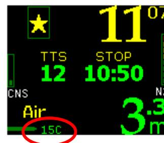
Keep in mind that the temperature sensor is inside the KAON unit, so it can take many minutes for it to adjust to a rapid external temperature change.
