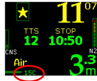
Keep in mind that the temperature sensor is inside the KAON unit, so it may take a moment for it to adjust to a rapid external temperature change.
