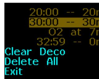
If you plan to dive a multi-level dive with different mixes for each level, you will need to set a “Switch” waypoint to tell your KAON to plan a gas switch. Let’s say that after 20m for 20 mins breathing 32% nitrox, you would like to spend 10 minutes at 40m (ca. 130 ft) and would like to breathe Air there. Then you would set up two “Normal” waypoints, and add a “Switch” waypoint:
