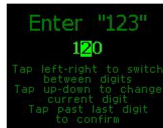
To unlock, just select “UNLOCK” by tapping on the side of your unit. You will have to enter the unlock sequence. It is also “123” and you input it in the same way as you input your PIN number. The screen will also remind you how to perform the unlock sequence. The unlock sequence prevents random unlocking of the unit – it is very improbable that random shakes will input that sequence.
