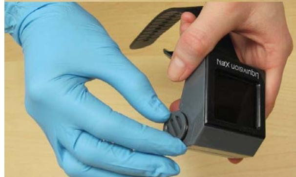
**6. Place the battery cap aside, on its back**
