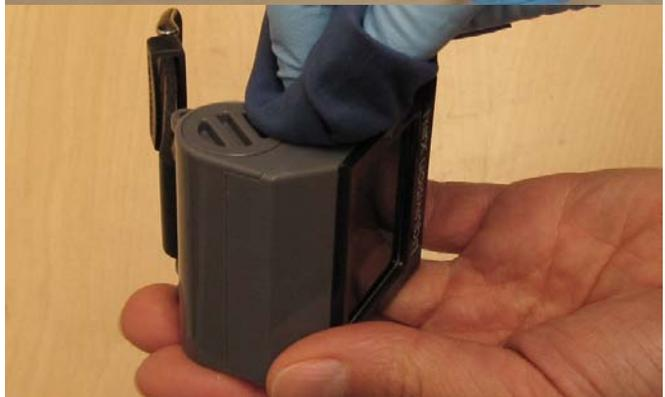
**4. Unscrew the battery cap with a coin**
