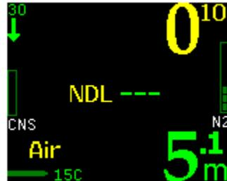
Velocity off or not ascending/descending      Velocity on – descending at 30mpm (current units - metric)
