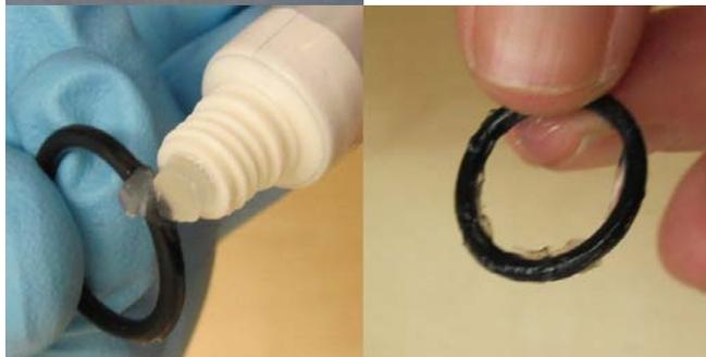
**16. Ease O-ring onto battery cap**
