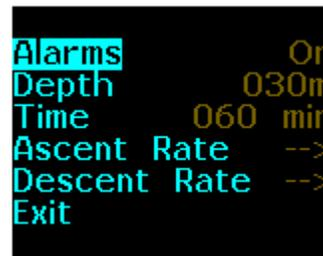
When the alarm is activated for any parameter, that piece of information will start blinking on your screen for one minute. If you do not correct the situation within one minute, the parameter display will invert (i.e. it will appear as black letters on colored background) until you correct situation causing the alarm. Once you do that, the alarm will turn off.
