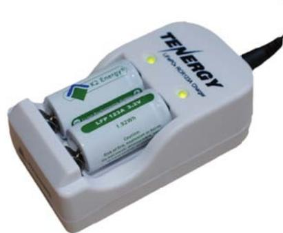
**DO NOT** use the old, black battery charger that was compatible with the Green ICR15340 batteries. Those batteries were Lithium Ion (Cobalt) and used a Lithium Ion (Cobalt) charger. This black charger will not charge your LFP batteries properly and **may damage them**.
