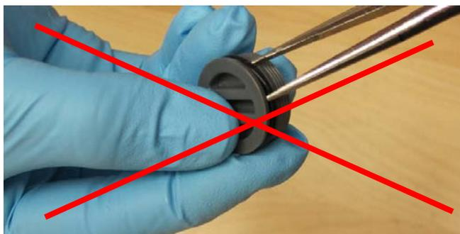
**14. Inspect the new O-ring for dust or defects**
