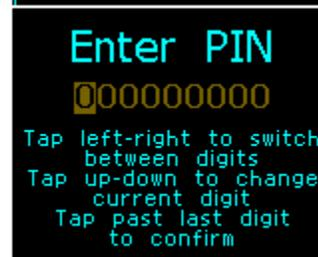
6. Tap Up or Down to change the first zero to the first digit of your PIN code. Tapping Up will bring the numbers 1-2-3-4-5... in sequence. Tapping Down will bring the numbers 9-8-7-6-5.... in sequence.
