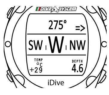
The electronic compass is able to correct the direction indicated for a tilt angle up to 85°.
