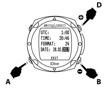
Pressing the **A** button the cursor place of EXIT by pressing the **B** button to confirm the setting returns to the clock function.
