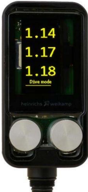
**Power-On:** Press the ENTER button two times within one second.
