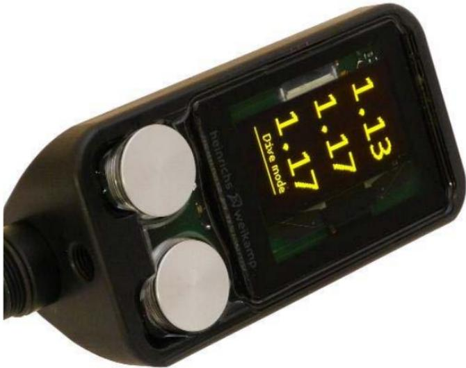
The ppO<sub>2</sub> Monitor allows monitoring of up to three O<sub>2</sub> sensor cells for rebreather diving (CCR/SCR/pSCR). Values are displayed on an OLED screen using a large font with high contrast. Optional, the values are output on a hWHUD display using (configurable) blink codes.
