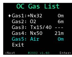
Use **gas setup** to configure presets for up to five gases for scubadiving as well as bailout gases for rebreather diving . You can switch between these presets when you change your gases while diving.
