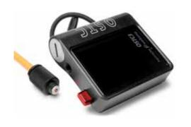
heinrichs weikamp delivers the OSTC3 ready for use with a high quality lithium battery (Saft LS14500). If the OSTC3 has not been used for a long time (more than one year), it may be necessary to replace the battery first.
