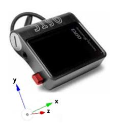
OSTC3 has a tilt-compensated electronic compass. Like all other electronic compasses it must be calibrated before use. The calibration compensates aberration that can be caused by the battery.
