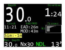
Change diving depth: In the simulator you can also change the depth while the dive computer is in dive mode. Push repeatedly SET/MENU to get into the depth menu. Select the desired value with SET/MENU and confirm with ENTER.
