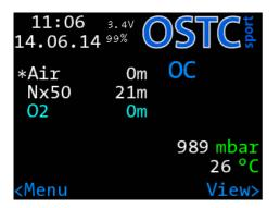
In surface mode the display shows general information as time, date, temperature, ambient pressure and battery status. After a dive the display also shows tissue saturation and the no-fly-time.
