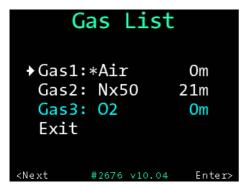
The presets are marked like this: **Air** for compressed air (21% oxygen) and **Nx** for Nitrox (e.g. a mix of Nitrox 31 is shown as Nx31). 100% oxygen are shown as **O2**. If the oxygen value is lower than 21%, there will be the warning **Err**. This gas mix is unusual.
