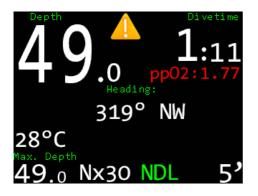
Warnings appear permanently on the display. Up to two warnings are shown simultaneously. If there are more than two warnings, the warning display toggles every two seconds. If there are critical warnings, a yellow warning sign is displayed additionally. Warnings are shown for the following items:
