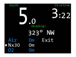
In the menu **gaslist** you can make your gas change and select the actual gas. You can choose the gas mixes that you prepared in **gas setup** in the surface mode. The actual gas appears on the main display.
