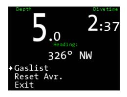
In dive mode (**OC**) you can select your preset gases (**gaslist**) und reset the calculation of your average depth (**reset avr./stopwatch**).
