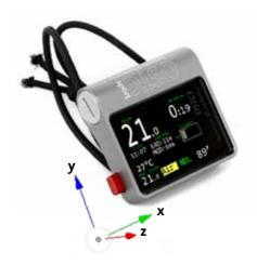
OSTC sport has a tilt-compensated electronic compass. Like all other electronic compasses it must be calibrated before use. The calibration compensates aberration that can be caused by the battery.
