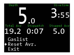
In dive mode you can select the average depth and stopwatch with the right button. **Total avr** indicates the average depth since the start of the dive. **Stopped avr** indicates the average depth for a period of time that you choose.
