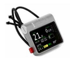
heinrichs weikamp delivers the OSTC sport ready for use with a high quality lithium battery (Saft LS14500). If the OSTC sport has not been used for a long time (more than one year), it may be necessary to replace the battery first.
