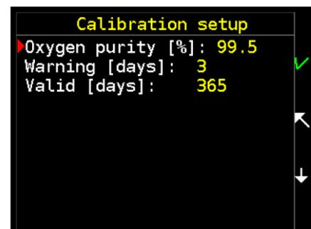
setpoints. At the end of its service life, an oxygen sensor can successfully undergo calibration to 21% (air), but will no longer be capable of measuring pO<sub>2</sub> of 1 bar or higher.
