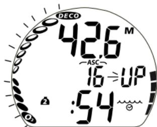
Fig. 65 – ÉCRAN PRINCIPAL DE VIOLATION AVEC LIMITATION AU MODE PROFONDIMÈTRE
