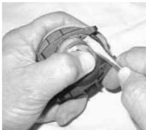
Fig. 102A – MISE EN PLACE DU CERCLAGE DU COUVERCLE
