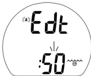
Fig. 22 – RÉGLAGE ALARME DE TEMPS ÉCOULÉ (EDT)
