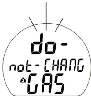
Fig. 72 – ALARME – NE PAS CHANGER DE GAZ
