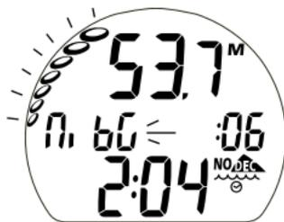
Fig. 94 – ALARME DE BARRE GRAPHIQUE DE L'AZOTE EN MODE FREE (pendant signal sonore)
