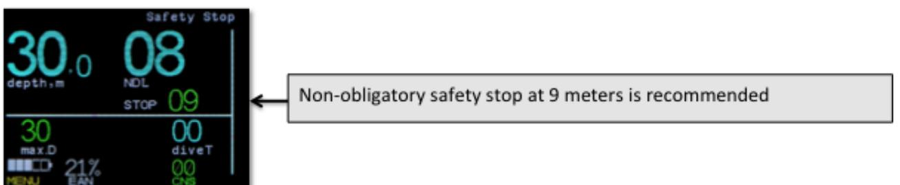
When reaching the safety stop depth, safety stop countdown timer will automatically switch on.
