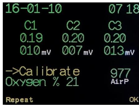
When calibration is finished, press **OK** to save, or, if required press **Repeat** to repeat.
