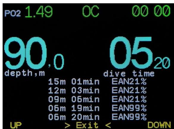
A list of forthcoming safety stops is in the bottom part of the screen. To browse through the list use buttons **Up** и **Down**. Exit from browse display - simultaneous pressing of 2 buttons.
