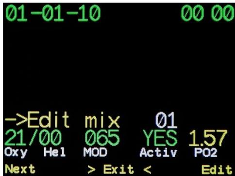
Navigating between fields is made with  $\rightarrow$  button, changing the field value is made with  $+$  button. **MOD** field value is taken into account when best mix is offered at the moment of gas change via **->selectmix** menu item, and when TTS value calculation and when planning your dive.
