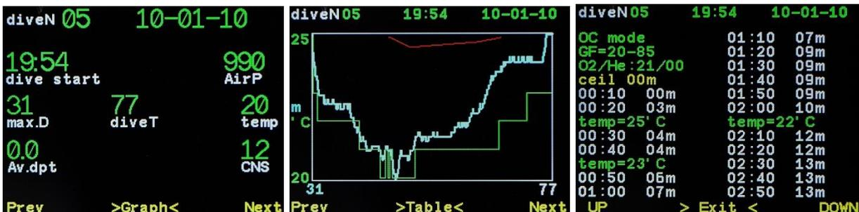
Switching between modes is done by simultaneous pressing of 2 buttons.
