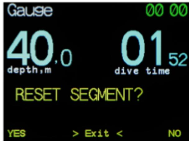
Average depth and current segment time can be reset by one pressing of the button with further confirmation
