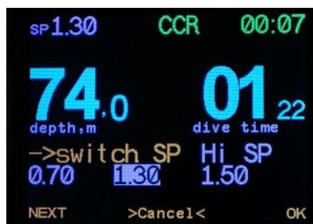
manual switching between Low, High and Deco Setpoints. Choose the required Setpoint with button **Next** and confirm with button **OK**.
