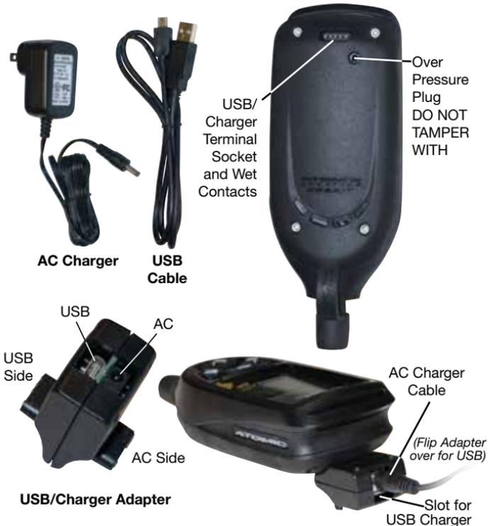
**NOTE:** Always unplug the adapter from the Cobalt when not charging or the battery will discharge.
