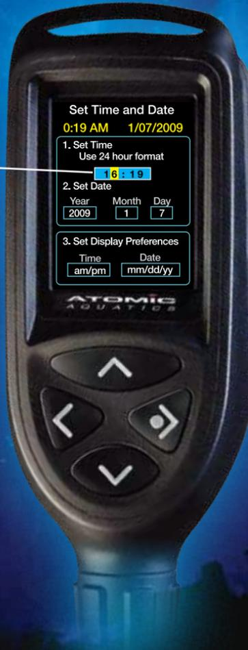
Important! The time and date must be correctly set in order to accurately track your dives. Setting the time and date enables the Cobalt to keep track of dives chronologically. The internal clock is also used for decompression calculations. If you travel to a different time zone, set to the local time before diving.
