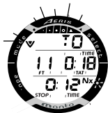
Fig. 83 - DELAYED VIOLATION #1 MAIN
