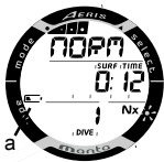
Fig. 3 - LOW BATTERY WARNING
