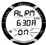
Fig. 21 - DAILY ALARM STATUS
