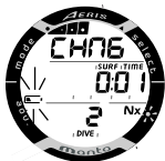
Fig. 4 - LOW BATTERY ALARM
