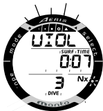
Fig. 87 - VIOLATION GAUGE SURFACE
