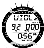
Fig. 86 - VIOLATION GAUGE MAIN
