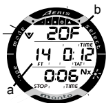
Fig. 82 - CONDITIONAL VIOLATION MAIN
