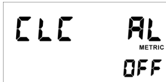
Figure 41a PROGRAMMING MODE (Clock Alarm - On/OFF)
