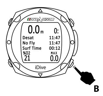
Once on the surface and 10 minutes has elapsed, by pressing the **B** button, you will see some important post-dive data as:
