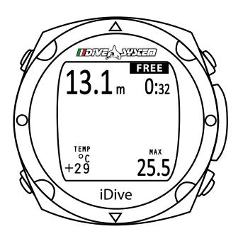
Pressing the **B** button the display will show the temperature of the water on the left and on the right the maximum depth reached during the entire session dive.
