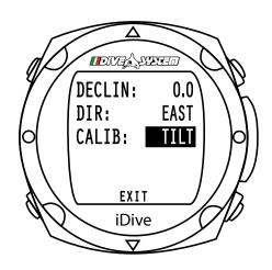
Rotate around the longitudinal axis until no signal appears OK as showed in the picture.
