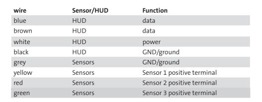
The HUD is digitally controlled by the four wires of the electronic box mentioned in the overview. The high flex cable out of the HUD has four wires only. The colors of the wire are identical to those of the cable from the electronic box.
